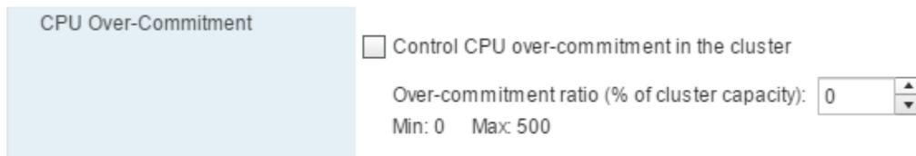
The screenshot shows a configuration panel for 'CPU Over-Commitment'. It includes a checked checkbox for 'Control CPU over-commitment in the cluster'. Below this, there is a numeric input field for 'Over-commitment ratio (% of cluster capacity)' with the value '0'. The minimum and maximum values are indicated as 'Min: 0' and 'Max: 500'.
